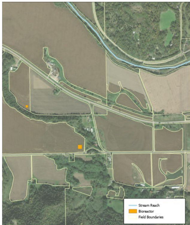
Figure 6. Outputs from the Bioreactor Tool. The small orange polygons are the potential bioreactor locations.
